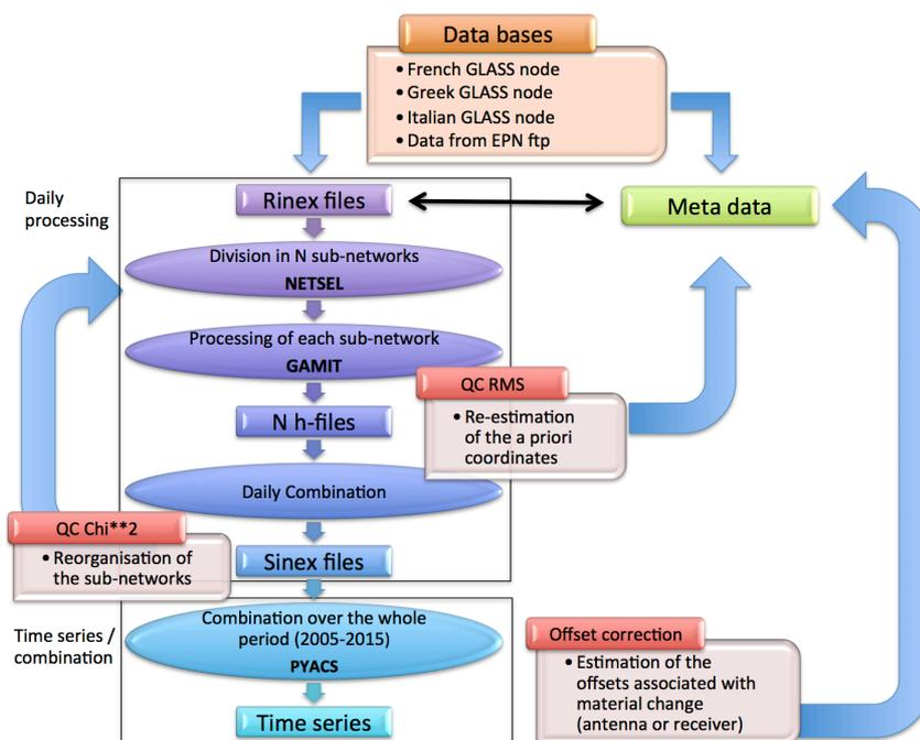
Figure 1: Processing chart at CNRS-UGA to produce time series
