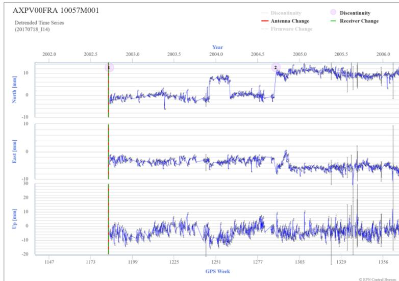
**Figure 3: Station AXPV00FRA: raw detrended position time series between 2002 and 2006.**
