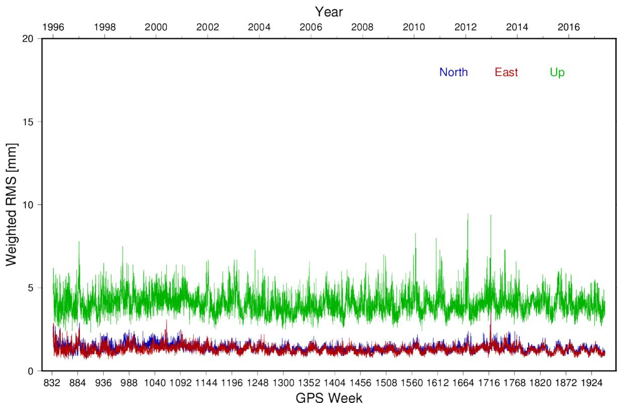
**Figure 1: Time series of the weighted RMS (North, East and Up values) of the cleaned daily combined EPN SINEXs with respect to the multi-year combination.**
