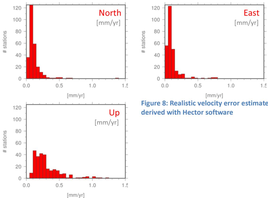
Figure 8: Realistic velocity error estimates derived with Hector software
