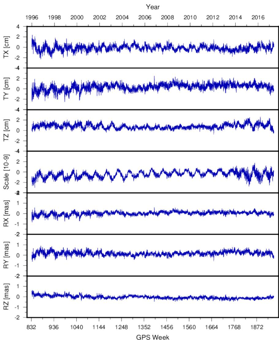
**Figure 2: Transformation parameters between the input daily combined EPN SINEXs and the EPN multi-year SINEX output of the combination. These 7 parameters show the reference frame alignment of the daily combined EPN SINEXs with respect to the EPN multi-year solution**
