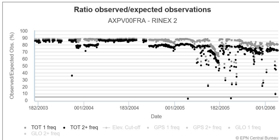
**Figure 4: Time series of the ratio observed versus expected RINEX observations between summer 2003 and 2006 at AXPV00FRA.**
