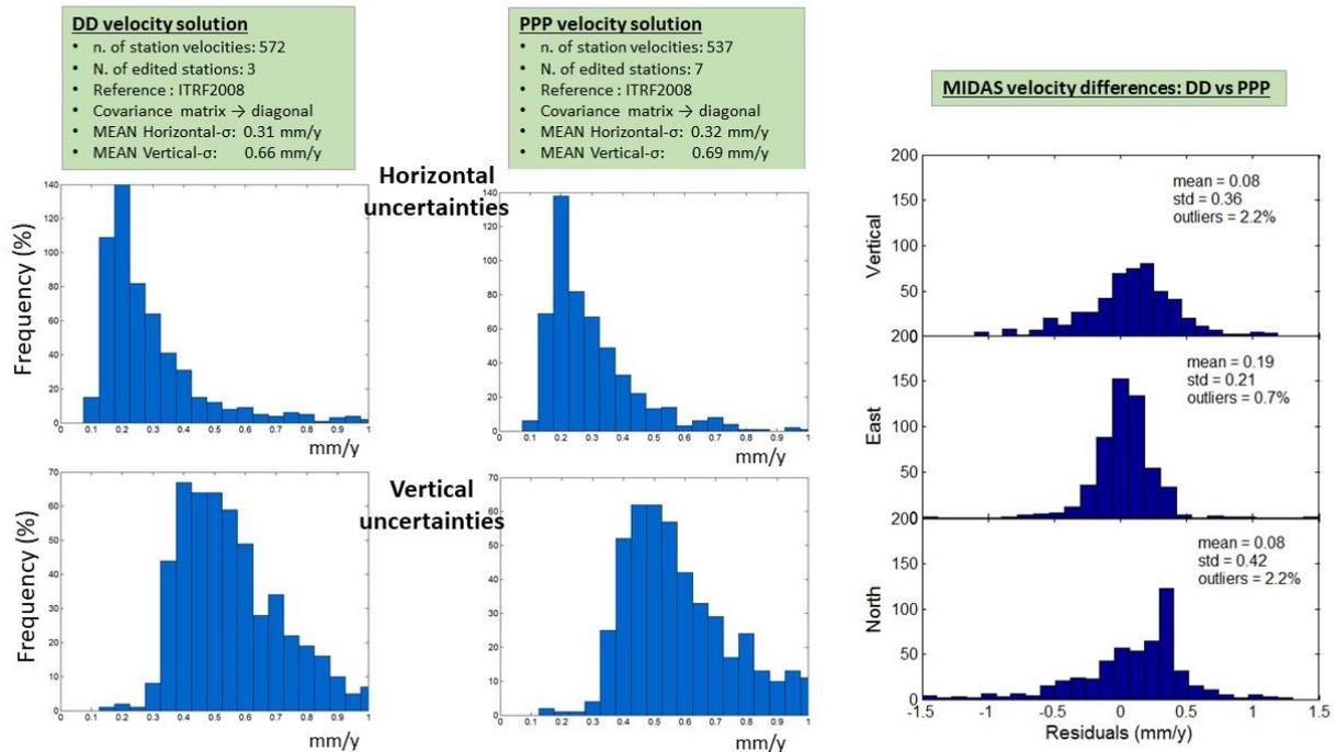
Figure 1: Distributions of horizontal and vertical uncertainties for both the DD and PPP velocity solutions (left and centre) and statistics on their differences
