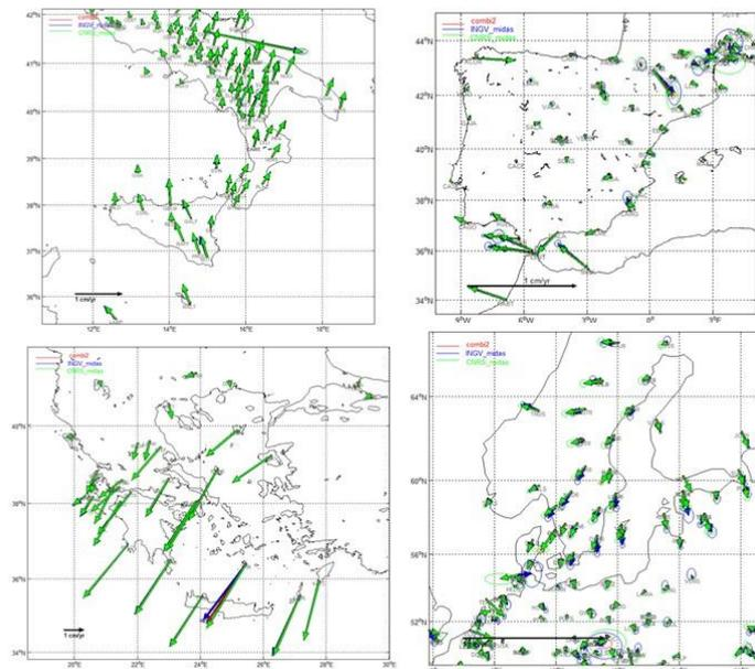
*Figure 5: Spatial comparisons between COMBI (red vectors), DD (green vectors) and PPP (blue vectors) velocity solutions in both slowly and quickly deforming regions*
